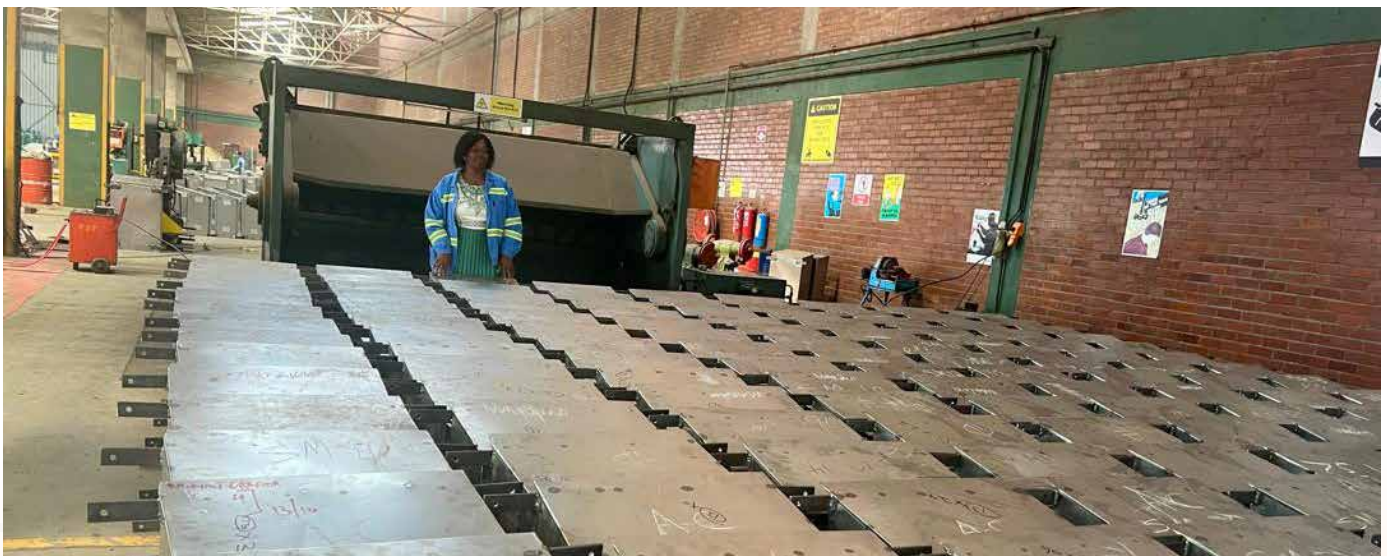
Batch of completed 2 door cubicles awaiting painting
